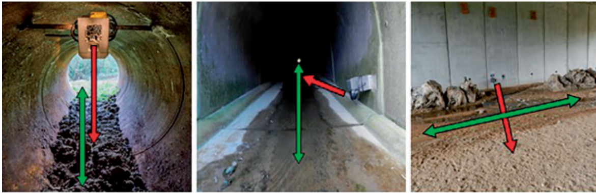
Figure 57: Possible orientations of camera traps (in red) with regard to targeted pathways (in green). a) positioned "above", in the axis; b) positioned "at an angle", on one side; c) positioned "perpendicular" to the pathway.
